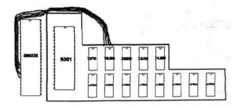
**KEMPSTON** - Produced a Centronics card to fit in the ROM port. The tiny bit of code is in EPROM but there is no provision for fitting a larger one to hold this code and TK2. The later MIRACLE Gold Card prevents the Kempston card functioning correctly as it interferes with A0 address line.
