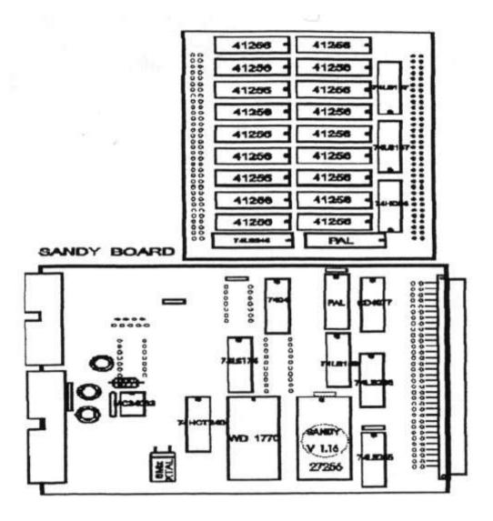
**SANDY** - This SANDY produced board is probably of earlier origin as it uses the TMS 4500 memory controller chip. Again this has a parallel printer port.
