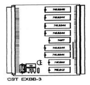
**INTERNAL** - To avoid bits hanging out of the end of the QL, several manufactures produced an internal 512K memory expansion upgrade. Here is the solder in CST version.
