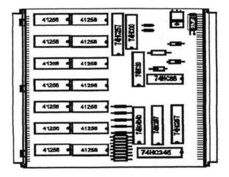
**TRUMP CARD** - The MIRACLE Trump Card is a disk interface combined with the provision for larger amounts of memory up to 768K. PALs are used to address the extra memory . A tiny extra board is needed if more than two disk drives are daisey chained. The Trey card was a Trump Card without the memory. Just sticking the extra memory chips in will not work as different PALs are needed. trump\_pic
