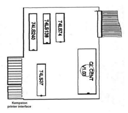
**TR SYSTEMS** - A disk interface with or without 128K of additional memory plus a parallel printer port. The additional holes on the board are probably to increase the memory size to 512K. I have not seen a full 512K version therefore have no knowledge of what chips are required. The ROM VI.12 has a peculiar early FORMAT routine doing 3 passes over the disk. Also it takes at least 3 tries to get a directory.
