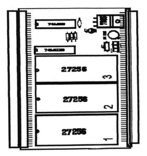
**TERRY HARMAN** with the help of others produced a similar board of slightly larger dimensions. This made extraction easier but there are problems in using ROMs other than JS or later. The easy hardware solution is to use fast logic chips. The essential access to the SP lines involves cutting tracks and soldering in wires.
