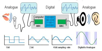
The minimum sample rate of any signal without introducing errors is twice the highest frequency present in the signal and is called the Nyquist frequency or Limit. A Digital representation can be expressed as a number of on/off's, high's & low's or in binary logic of 1's and 0's.
