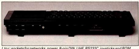
L to r: sockets for networks, power, 8-pin DIN, UHF, RS232C, joysticks and ROM
