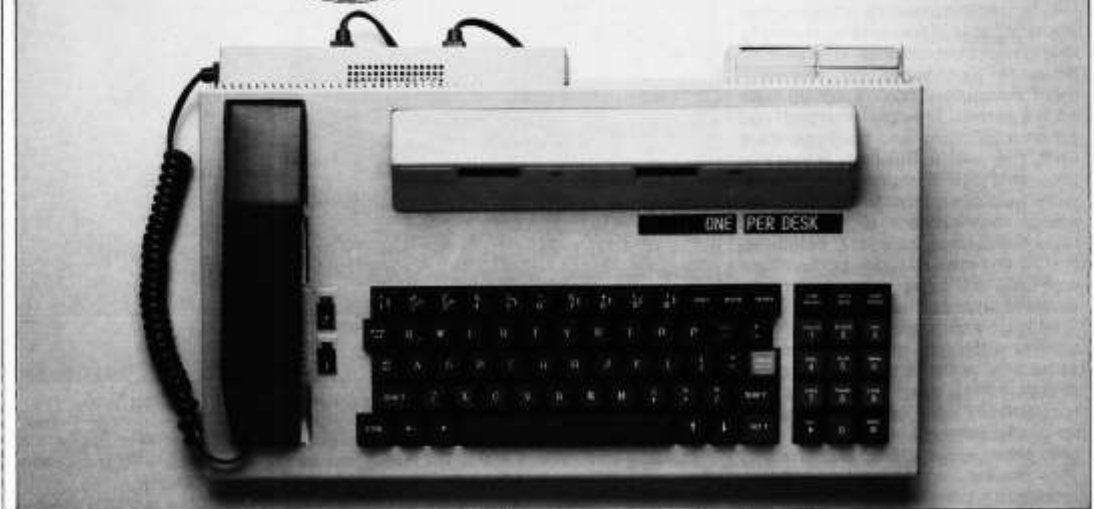
The standard qwerty keyboard incorporates a pair of microdrives and a telephone handset
