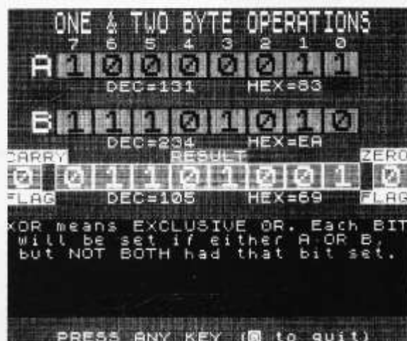
The picture shows how the MC Tutor explains the machine code XOR instruction. MC Tutor was featured in the June 1989 issue of the Spectrum tape-zine Network .
