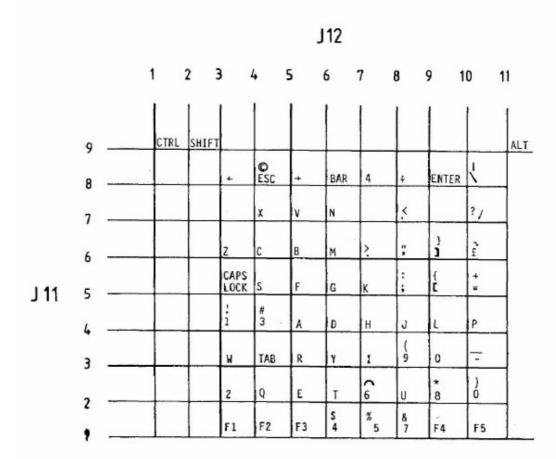
In fact this diagram is of the Black Box QL keyboard. At each crossing of a row and column there is a switch, which is a key of the keyboard. As shown below.
