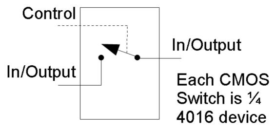
So there is no need for an excessive number of these devices, they have been arranged that one switch is required for each row and one switch for each column. There is a switch bus, so any two switches create the required crosspoint.
