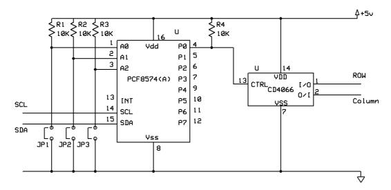
So connect the CD4016 to the required row and column and with the fact it is driven from a separate parallel device mean there is independent control of the this switch so we can "Press" two keys at the same time. By the way you can use either CD4016 or CD4066 devices they are the same for this type of application.
