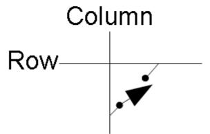
As you can see there are 65 keys on a QL keyboard, which would need at least 66 wires, one for each key plus say ground, however by using the scanning keyboard with row and columns only 20 wires are required.
